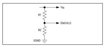
Figure 1. Setting the Input Undervoltage Lockout
