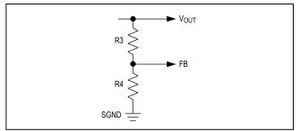
Figure 2. Setting the Output Voltage
